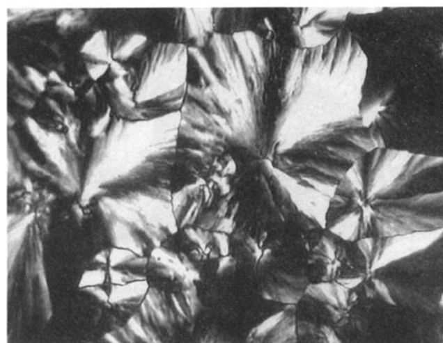
Figure 3. Virgin texture after fast cooling ( 20 \text{ K min}^{-1} ) from the isotropic liquid ( 10 \mu\text{m} ). Field of view c. 400 \times 300 \mu\text{m} .
